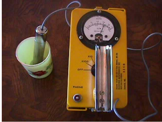
Picture 4: Radiation six times above background found in this piece of China.
