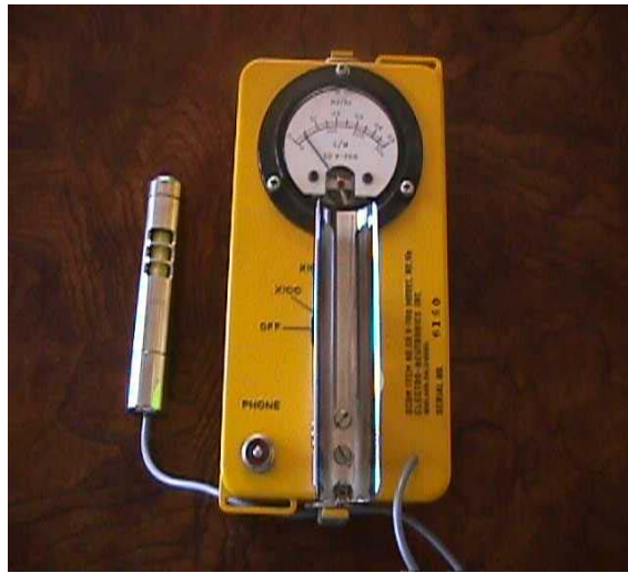
Picture 1: A V-700 Geiger counter measuring about .05 mR/hr background. Notice that the so-called beta window is open.
